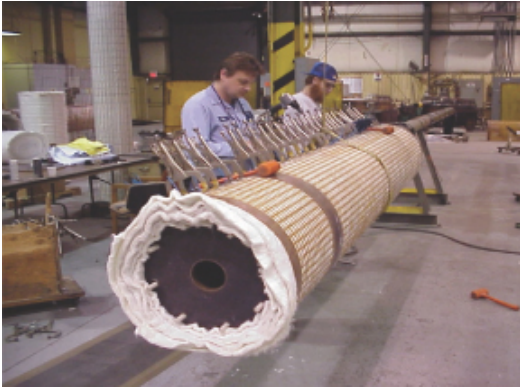
CECO Filters Fiberbed Filter Being Assembled
